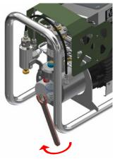
3. Replace crank oil cap. **Ensure to not over tighten** as this could damage the seal
